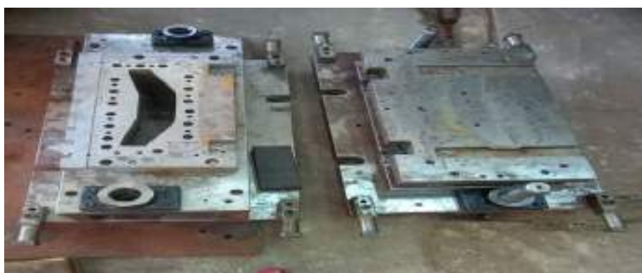
Press tool for Seat Belt Buckle for citroen india through M/s Preto tooling
